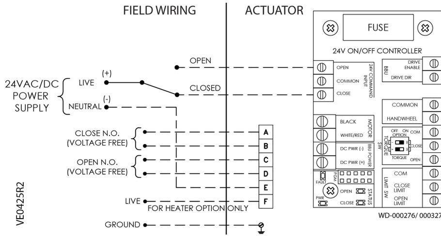
Figure 1. 24 Vac/dc On/Off Wiring 600 and 2000 lb.-in. Models.
