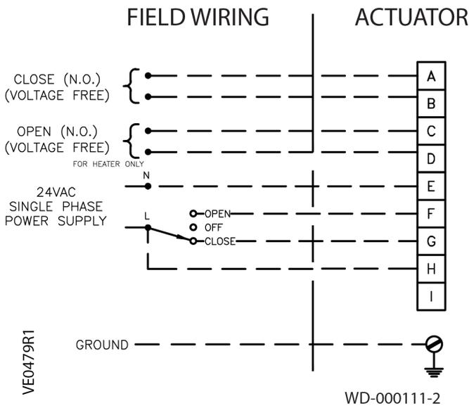
Figure 2. 24 Vac Wiring 5000 lb.-in. Models.
